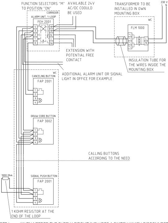
NOTE! WHEN NEEDED THE SUPPLY CIRCUIT INCLUDES A SWITCH WHICH DISCONNECTS ALL TERMINALS. THIS SWITCH MUST BE INSTALLED IN A PLACE WHERE UNINTENTIONAL USE IS PREVENTED
